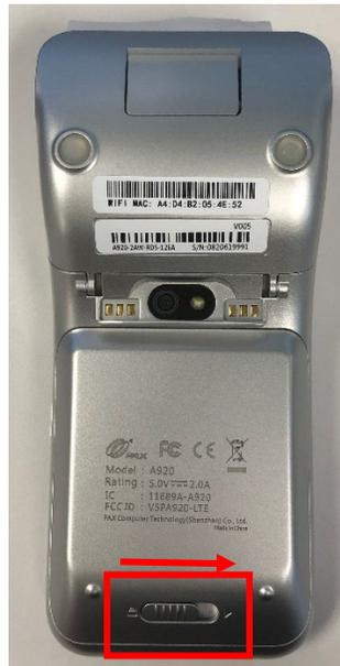
3. Lift and remove the battery cover. Once the cover has been removed, you can push up and pull out the battery.
