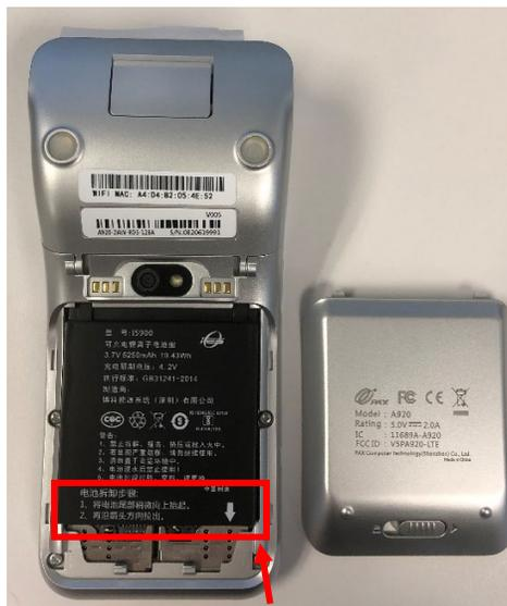
4. Set the battery aside in a safe location. To reinstall the battery, place the battery back in the battery slot and push up to secure it.
