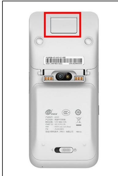
2. Install Paper Roll according to the diagram inside with the paper coming out from the top of the roll.
