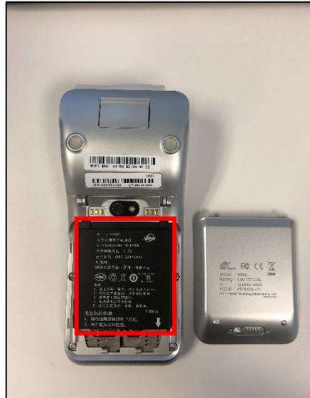
3. Insert the SIM card or Micro SD card (with adapter) into the card slot with the contacts facing upwards and the clipped corner of the card facing forward and to the right. Once the card is inserted, replace the mount cover and screw before turning the device on.
