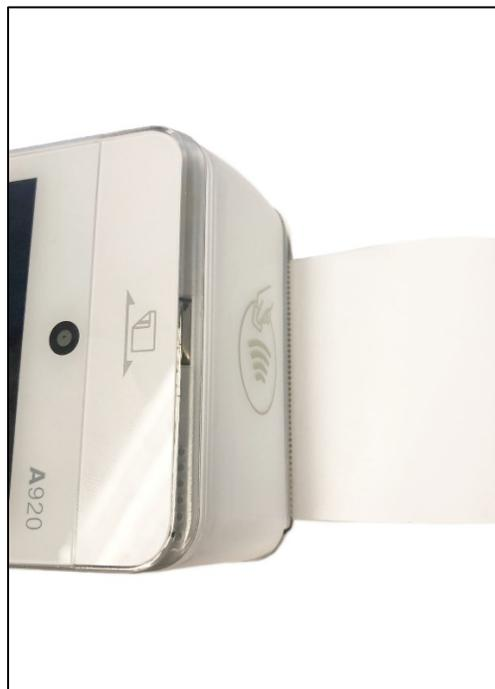
5. Firmly hold the paper and from an approximate 45-degree upwards angle tear the excess paper.
