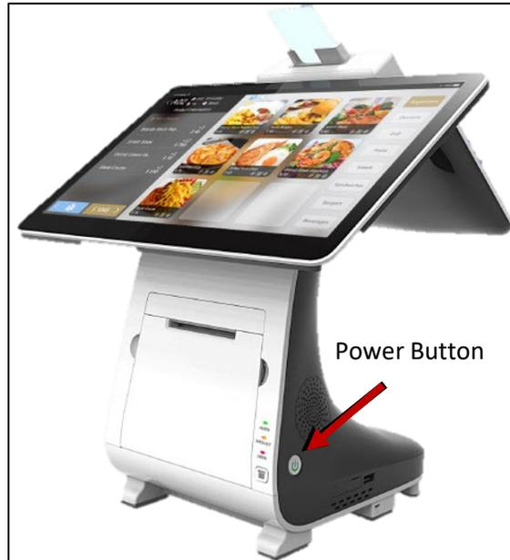
**Note:** If the power supply is not connected when the E800 is powered up, a message displays stating that you need to connect the power supply for the printer and printer-related ports to work properly.
