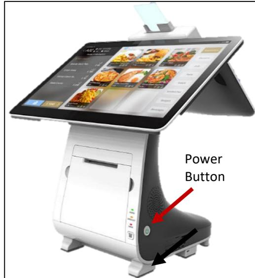
Press and hold the button for 3 seconds and the E800 will turn on.
